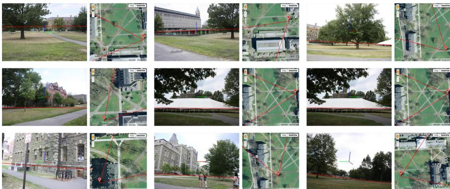
Fig. 3: *Sample estimated poses for the Quad dataset.* This figure shows a few images that were successfully registered, along with their estimate pose overlaid on a map. The annotations have the same meaning as in Figure 1. (Best viewed zoomed in.)
